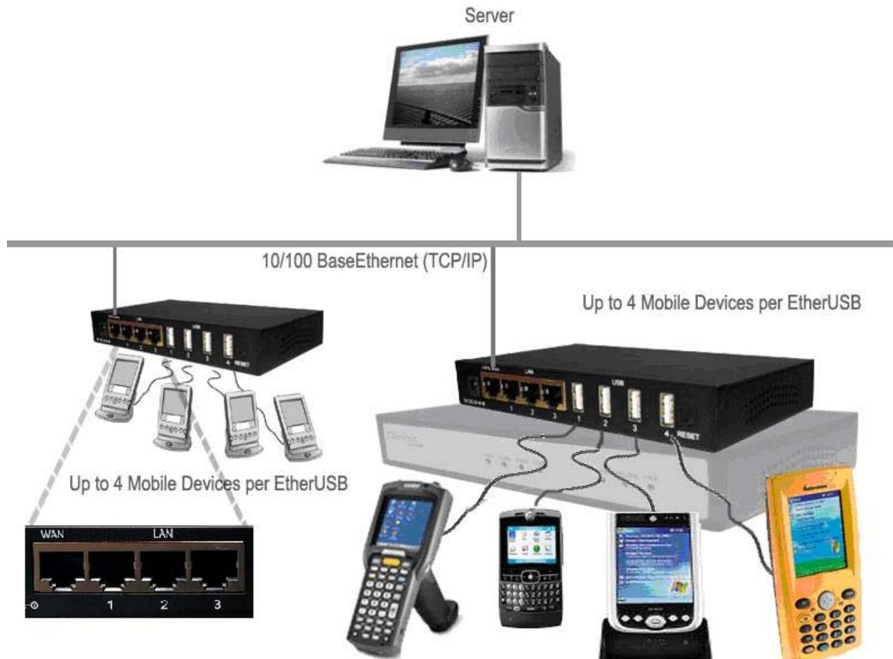
EA104 has four USB host ports that simultaneously connect up to four PDAs through their USB ports to an Ethernet network. Each connected PDA can perform server synchronization, Internet browsing, and file transfer.
