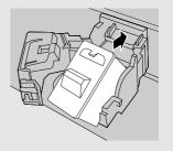
Place your index finger on the tab as shown and close the cartridge holder cover with your thumb. Make sure the cover clicks into place.
