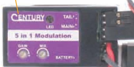
(For advanced users: Gain modifies gyro sensitivity. Mix modifies tail motor power)
