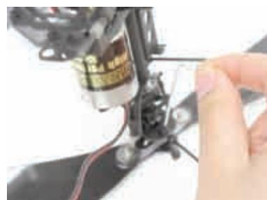
Flybar adjustment can be done by using a 1.5mm hex driver. The flybar should be equal length on both sides of the rotor head. An uneven flybar will cause vibration in the model making it more difficult to fly. After making any adjustment, make sure the flybar is tightly mounted.
