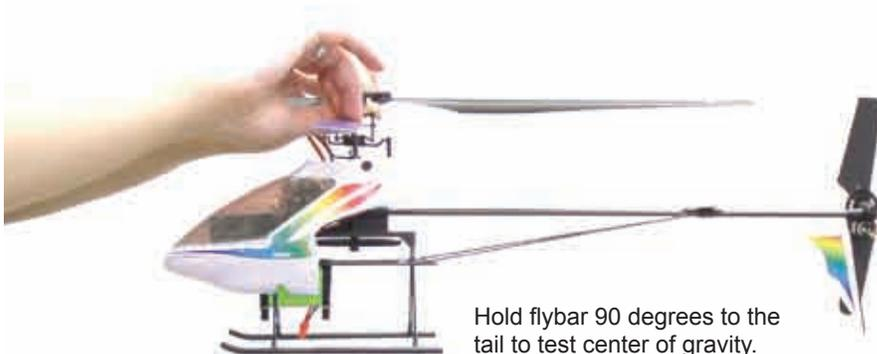
Hold flybar 90 degrees to the tail to test center of gravity.
