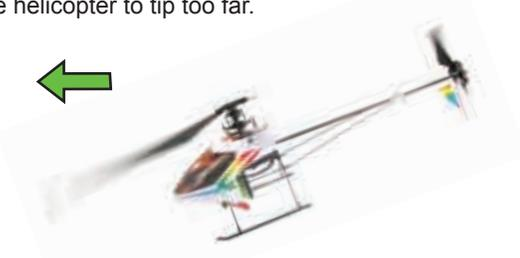
Helicopter tilts/drifts forward by adding upward Elevator input.
