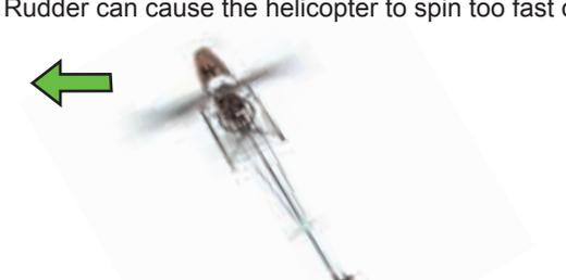
Helicopter nose moves left by decreasing the tail motor speed.
