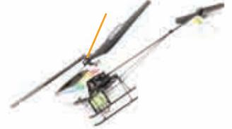
Aileron controls the helicopter's left and right tilt. This control will result in the helicopter drifting in the direction the stick is moved. Be careful! Too much Aileron can cause the helicopter to tip too far.
