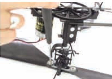
Blade tension can change after a few uses. The blades should be held by their screws at about the same tightness. Adjust the screws to about the same tightness. The blades should not droop when the helicopter is sideways but they should be loose enough to fold back in a blade strike.
