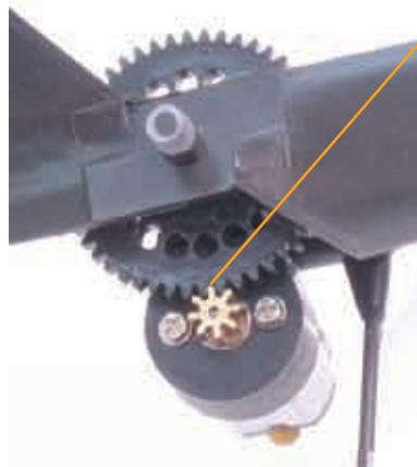
If the helicopter does not seem to turn properly or the tail motor seems to make a gritty sound as it tries to turn, check the gear mesh. If the gear mesh is too tight, this will cause excessive wear on the tail motor shortening its life and degrading performance. If the gear mesh is too loose, the tail will simply not respond well enough. Adjust the two screws that hold the motor in place in order to realign the mesh.
