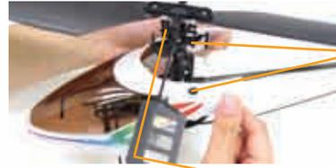
You may need to remove the canopy for some adjustments. Simply pull the rubber grommets off of the mounting rod.
