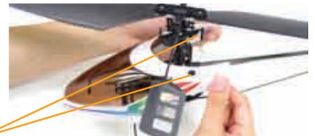
Replace the canopy using the two rubber grommets and mounting rod. **Do not obstruct servos while remounting the canopy!**
