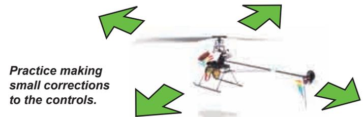
Only slight inputs are needed to move the helicopter. Too much input can cause the helicopter to tip too far to one side. Continue to make small corrections to keep it level.
