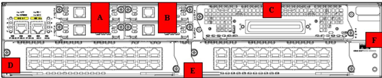
**Figure 5 – 2851 Tamper Evident Label Placement (Back View)**
