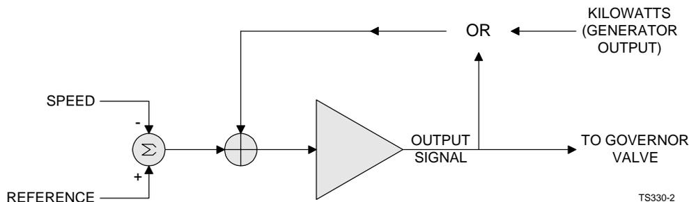
Figure 4. Droop-On-Output Or Droop-On-Kilowatts
