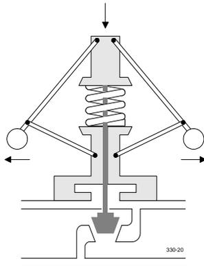
In this figure, centrifugal force of the flyballs is high enough to partially depress the spring and close the governor valve about halfway. Observe that turbine speed will stabilize at some RPM higher than that required to just barely compress the spring.
