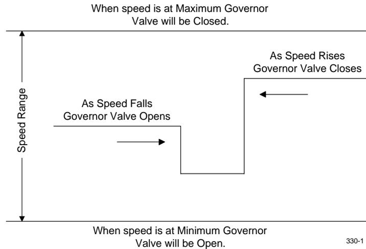
**Figure 3. Valve Open/Close vs. Speed Increase/Decrease**
