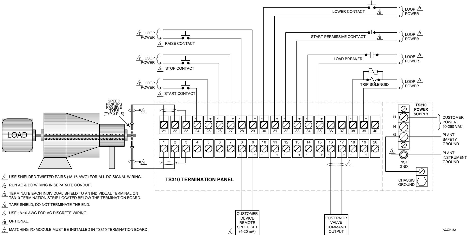
Figure 9. ACON.030 Wiring Diagram
