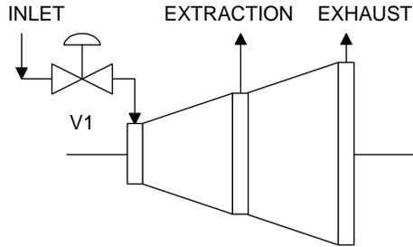
Steam is extracted from an extraction turbine.
