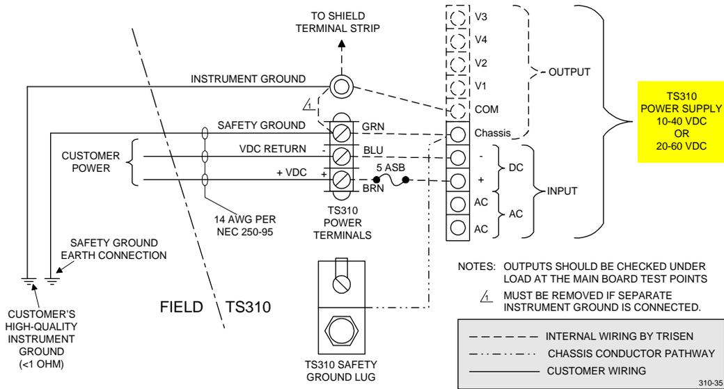
Figure 29. 10-40 VDC or 20-60 VDC Input Power & Ground Wiring
