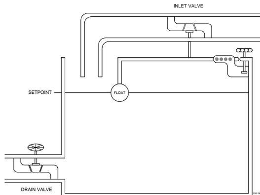
In this figure, the drain valve *D* has been completely closed. The inlet valve *I* will let water flow into the tank until the float *F* rises to the setpoint *S* (that level where the float causes valve *I* to shut off completely).
