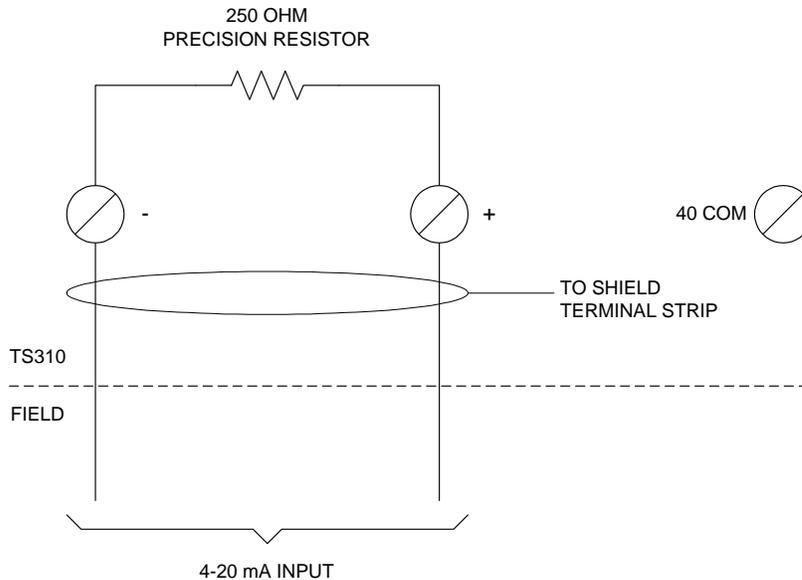
**Figure 21. Analog Input to External Power Wiring**
