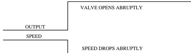
PIP DROOP provides short term stability based on the PI value (Proportional and Integral) while DROOP (the other P) is maintained independent of stability. With this control mode, DROOP settings of three or four percent are common and will furnish much more stable control of the turbogenerator.
