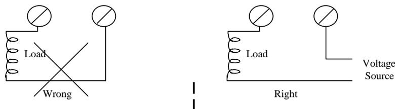
**Figure 17. Output Relay Module Wiring**
