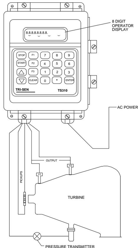
**Figure 15. Simplified Application Diagram**
