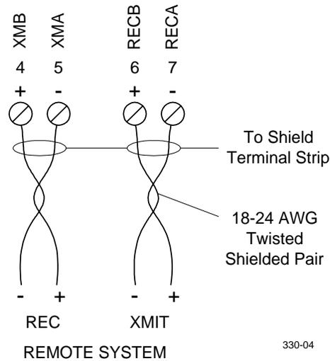
**Figure 23. RS422 Communications Wiring**
