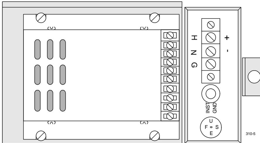
**Figure 6. TS310 Back View Showing Power Supply**
