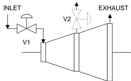
Extraction valve is usually inside the turbine, not mounted in the extraction line as shown here.
