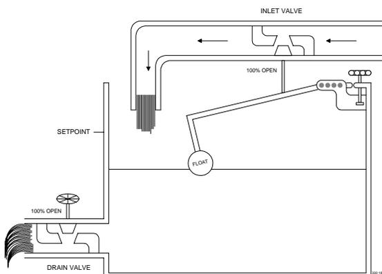
If the drain valve is now opened fully, the level will fall even more until the inlet water flow equals the outflow. The level (or measurement) will now stabilize at an even lower level, offset still further from the setpoint, as shown in this figure.
