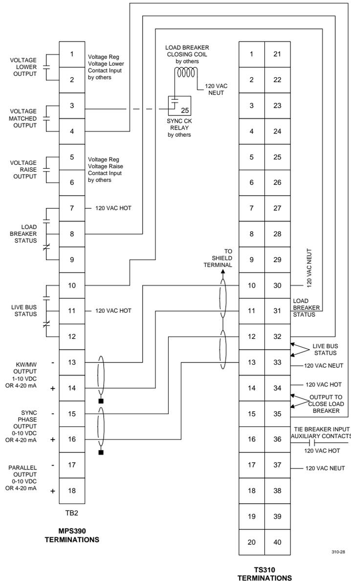
Figure 7. Minimum TS310/MPS390 Connections for Kilowatts and Autosynchronizing
