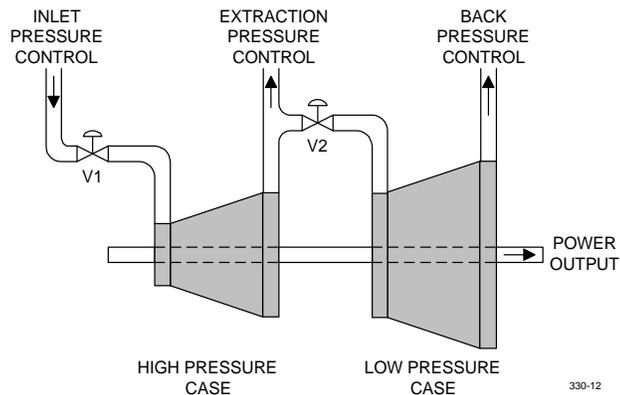
As mentioned above, only two of these variables can be controlled simultaneously since there are only two valves. Further, if one of the valves becomes limited, only one variable can be controlled. Priority entries determine which of the two will be allowed to control the turbine when this happens.
