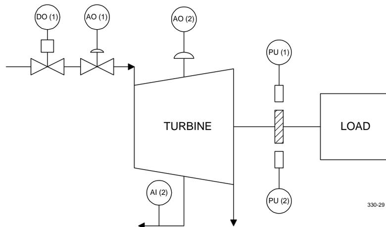
Figure 10. ACON.040 Speed/Load, Extraction Control Typical Application
