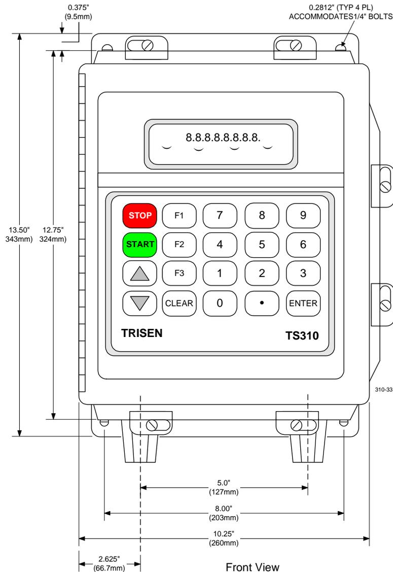
**Figure 10. Surface Mounting Dimensions, Front View**
