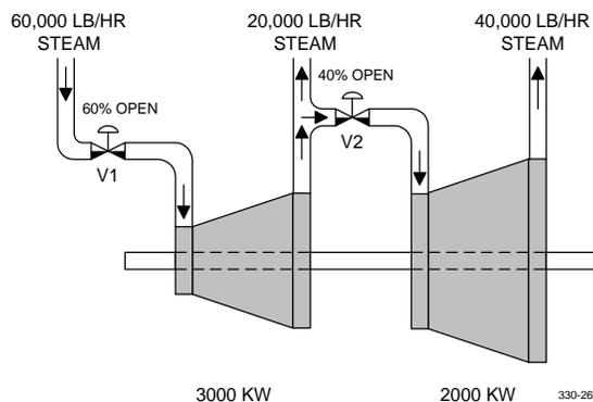
Thus, 20,000 lbs/hr of steam is now being extracted from the turbine to the intermediate steam header but total power is still 5000 kW. By following this pattern, the controller is able to increase (or decrease) the extraction steam flow without affecting power output.
