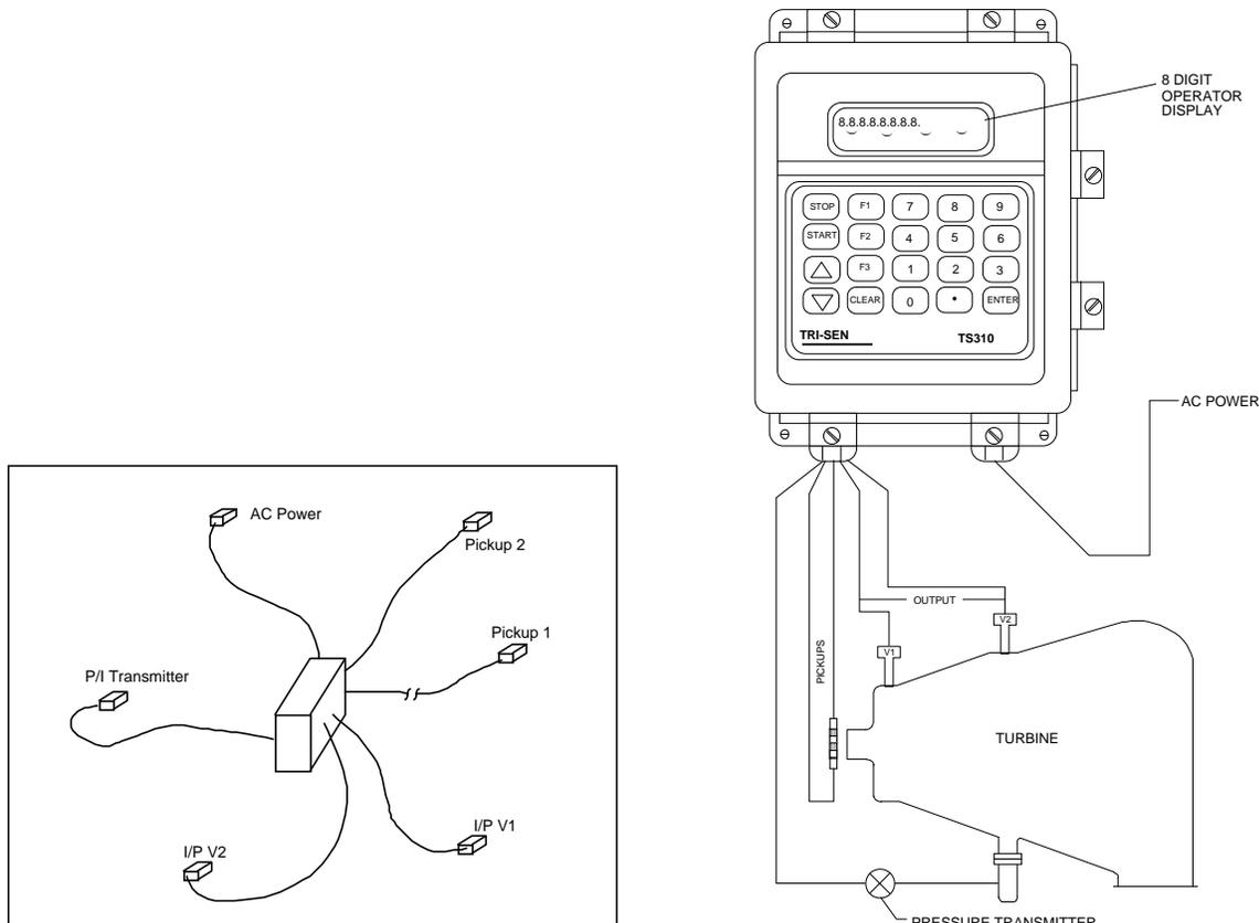
**Figure 14. Central Processor with Extensions**
