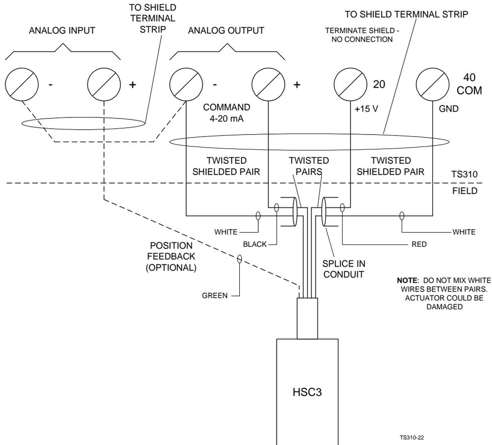
Figure 27. TS310 to HSC3 Hydraulic Actuator Wiring
