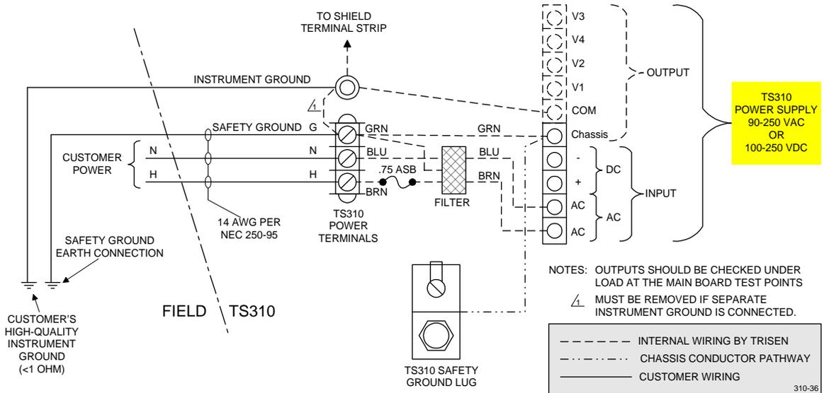
Figure 30. 90-250 VAC & 100-250 VDC Input Power & Ground Wiring
