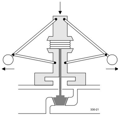
In this figure, centrifugal force of the flyballs has compressed the spring sufficiently to almost close the governor valve. (balls out) This would be a low load (high speed) condition where speed will keep the governor valve almost closed. If the load should increase, speed must fall. This in turn will cause the governor valve to open somewhat. RPM will then stabilize at a lower value.
