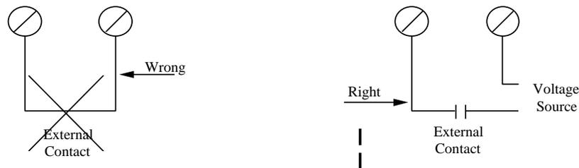
**Figure 16. Input Relay Module Wiring**
