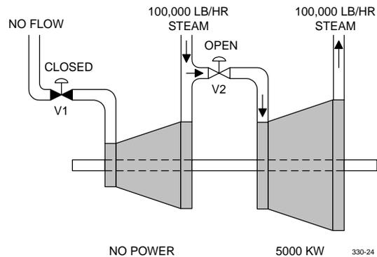
Both of the above examples are idealized fictitious situations since some *cooling steam* must always flow in each turbine case. In addition, we have not considered the amount of steam required to overcome friction, oil whorl and to drive turbine accessories. This can amount to 15 or 20% of the total steam consumed by the turbine and it produces no net power at the turbine coupling. However, the controller must account for this steam flow as well when controlling extraction turbines.
