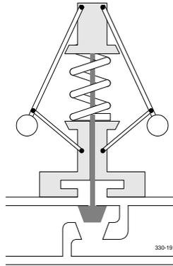
In this figure, we see a flyball governor at rest. The spring, which opposes the centrifugal force of the flyballs when turning, has forced the steam valve fully open. The valve will remain in this position until the centrifugal force of the flyballs reaches the level necessary to overcome the spring; it will then start to close the valve.
