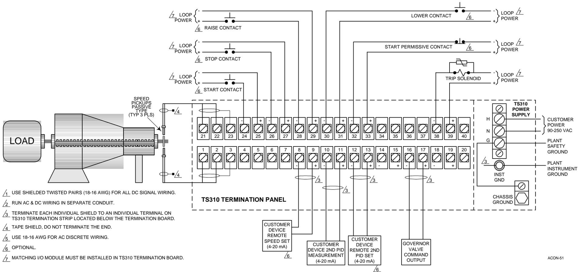
Figure 7. ACON.021 Wiring Diagram
