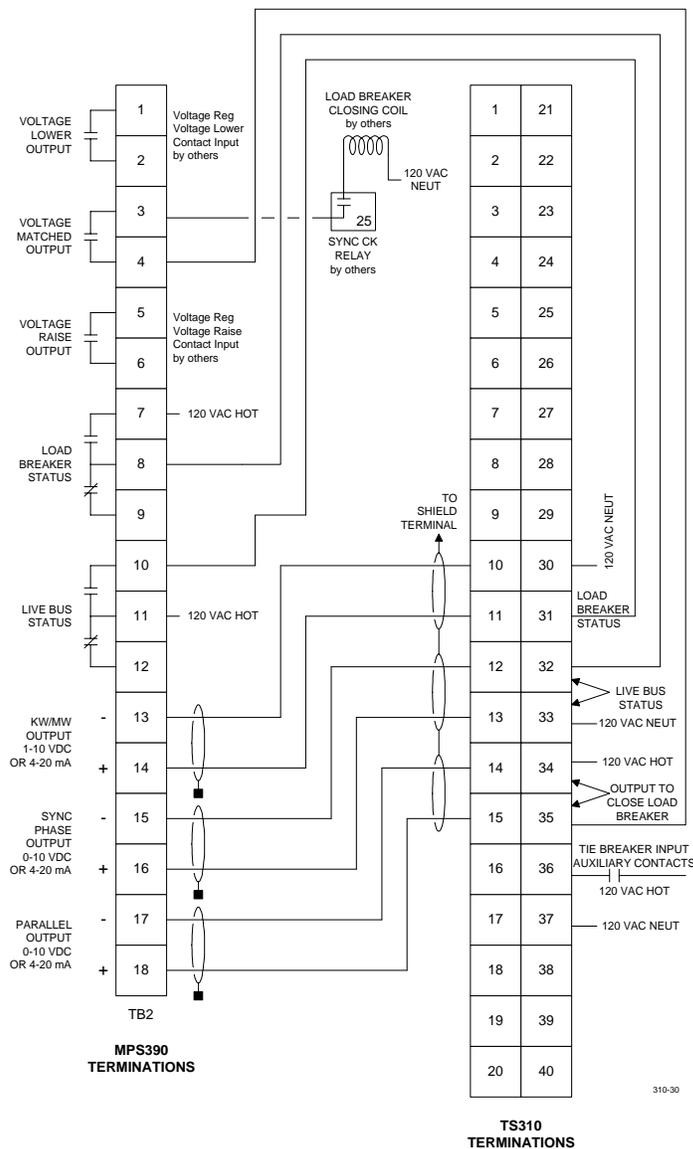
**Figure 8. *TS310/MPS390* Connections for Kilowatt Signal, Autosynchronizing, and Parallel Isochronous Operation**
