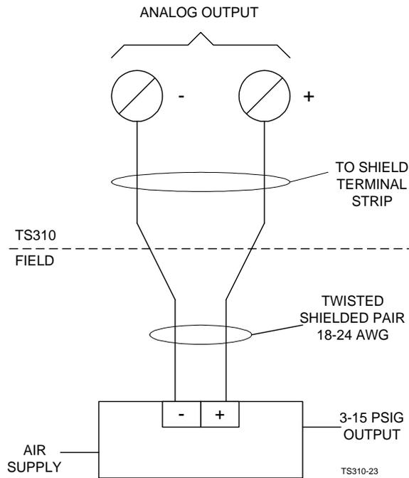
**Figure 28. Current to Pneumatic Transducer Wiring**
