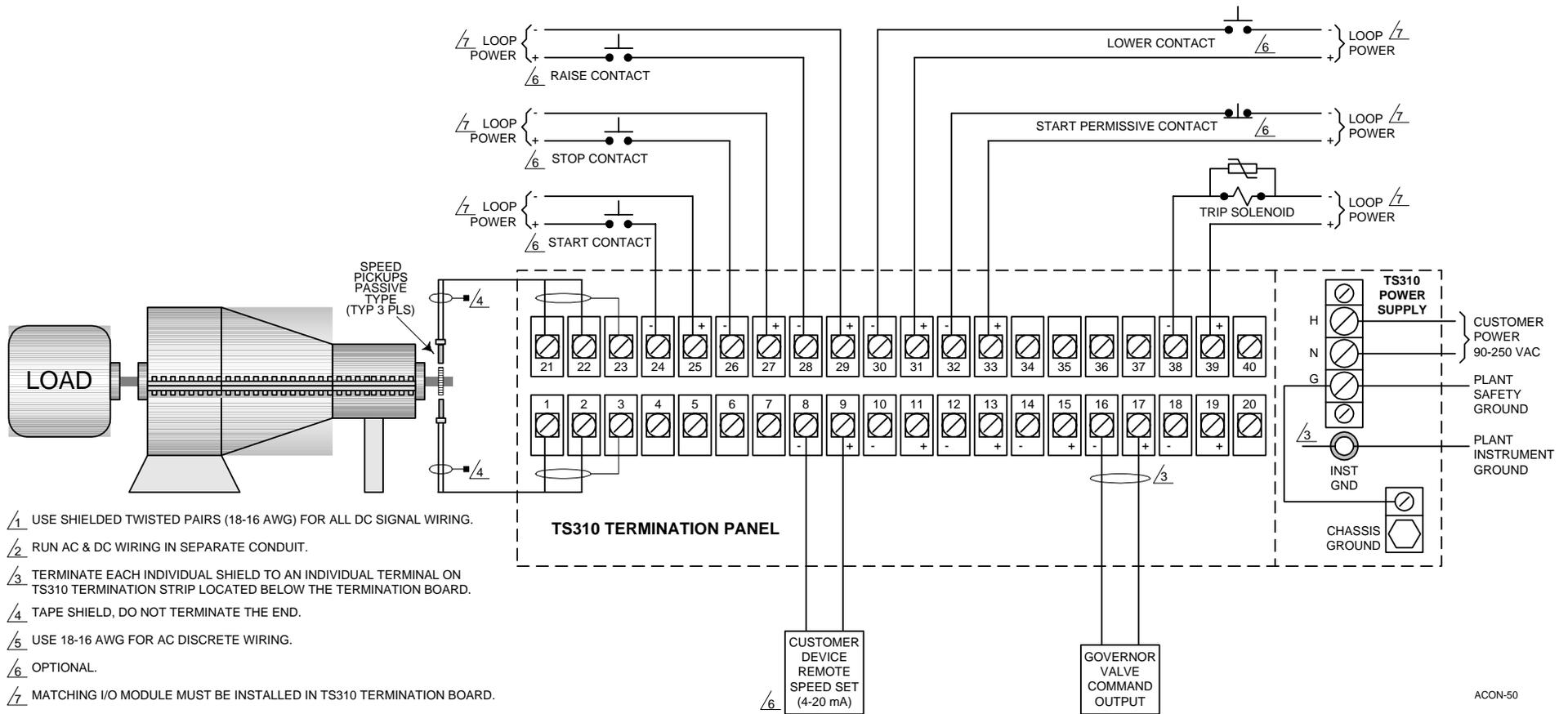
Figure 3. ACON.010 Wiring Diagram
