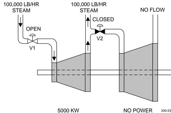
If V2 is open and V1 is closed, the LP case will produce 5000 kW from 100 PSI steam; 100,000 lbs/hr of steam will flow from the intermediate steam header; the HP case will produce no kilowatts; and no 900 PSI steam will be used.
