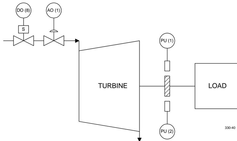
**Figure 2. ACON.010 Basic Speed Control Typical Application**
