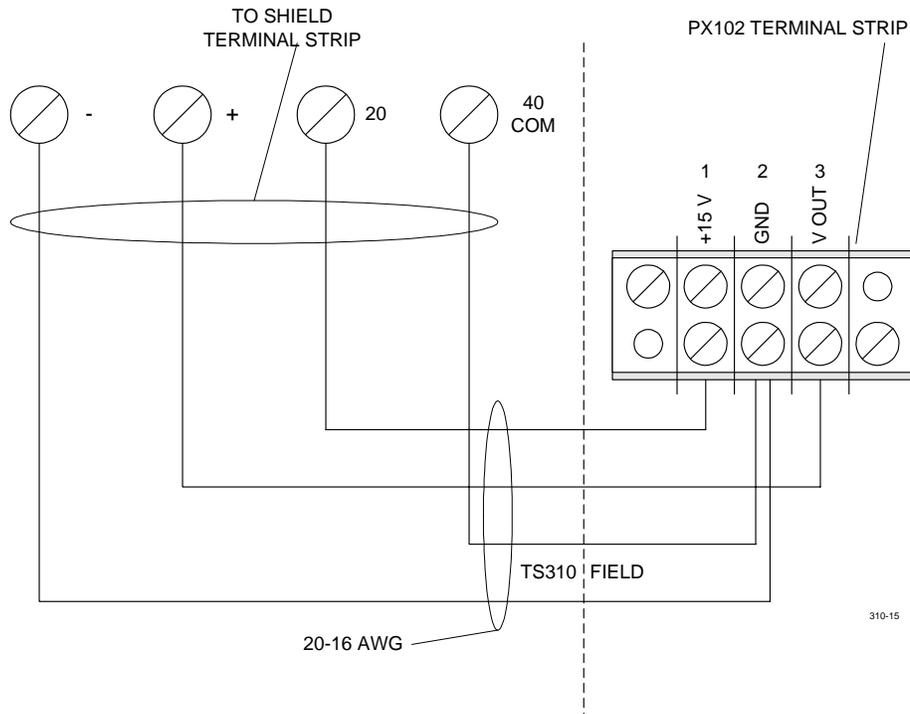
**Figure 20. *TS310* to PX102 Transmitter Wiring**
