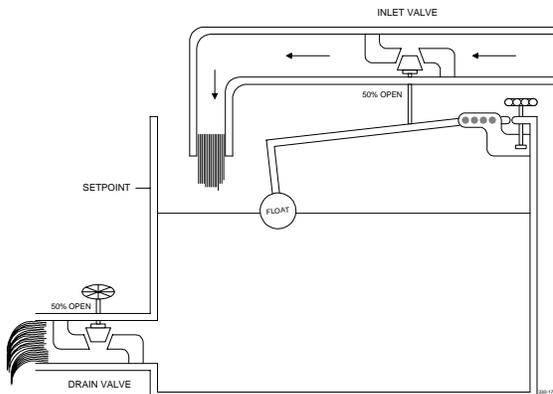
Now, if we partially open the drain valve *D* as shown in this figure, water will begin to drain from the tank. The float will begin to fall with the water level, opening inlet valve *I* until the volume of water flowing in exactly matches the volume flowing out, at which point the level (and float) will stabilize at some intermediate level below the setpoint.
