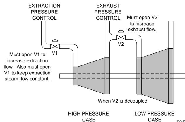
Conversely, it may be desirable to operate extraction pressure control and backpressure control simultaneously without controlling power output. In this case, decoupling V2 will operate as follows:
