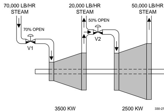
Thus, 20,000 lbs/hr of steam is still being extracted from the turbine to the intermediate steam header but the total power has increased from 5000 kW to 6000 kW. By following this pattern, the controller is able to increase (or decrease) power output of the turbine without affecting the extraction steam flow.
