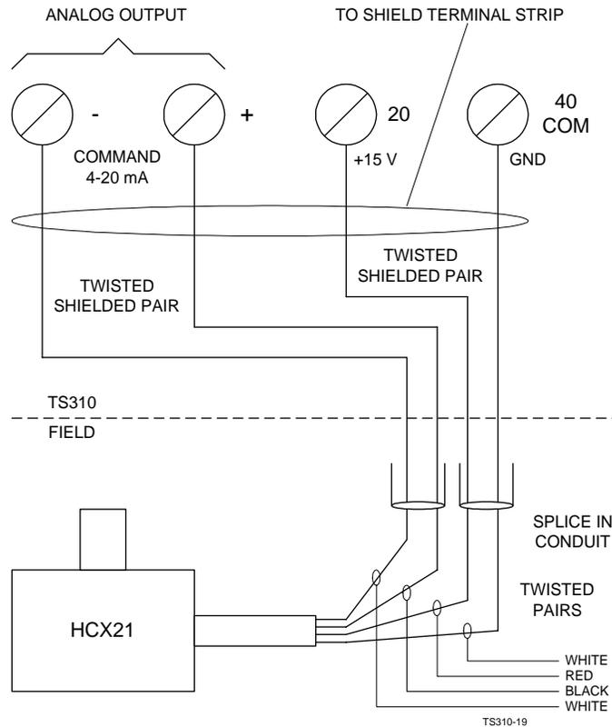
**Figure 26. *TS310* to HCX21 Transducer Wiring**
