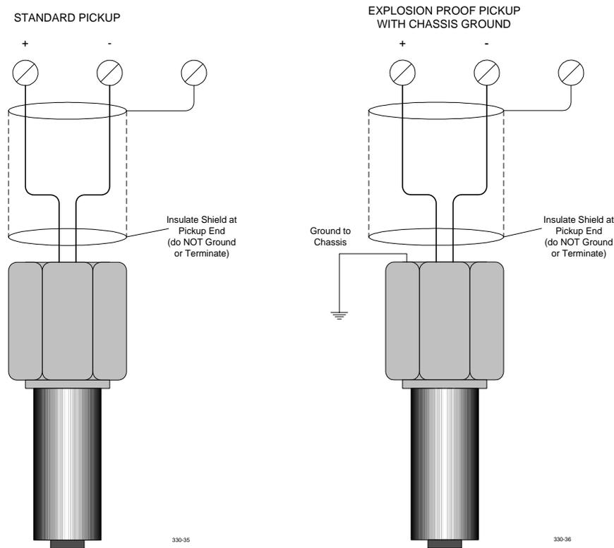
**Figure 24. Magnetic Speed Pickup Wiring**
