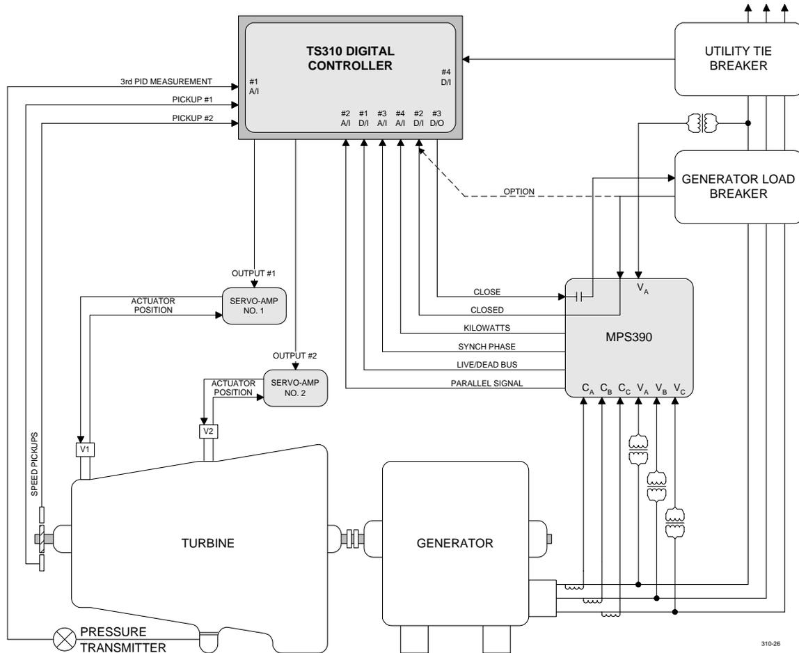
**Extraction Steam Turbine/Generator Application Including an MPS390**
