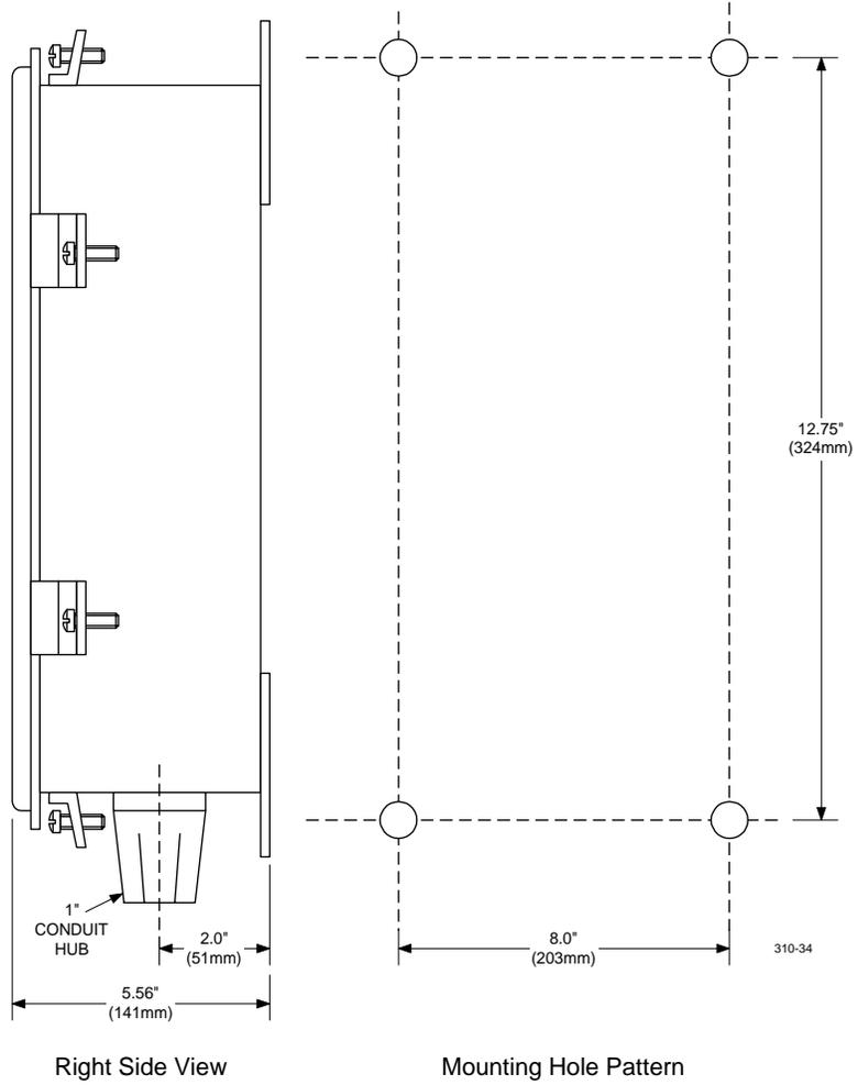
Figure 11. Surface Mounting Dimensions, Side View and Mounting Holes
