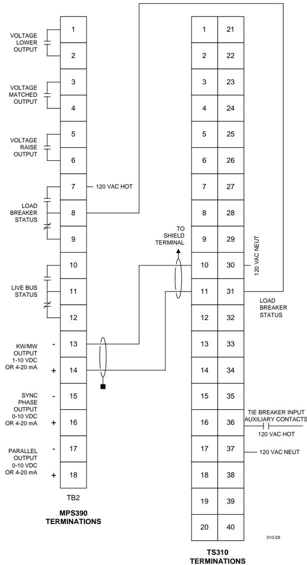
Figure 6. Minimum *TS310*/*MPS390* Connections for Generator Output (Kilowatts)
