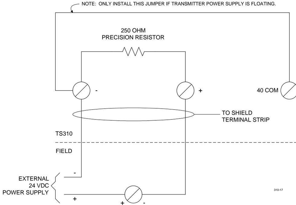
**Figure 22. Two - Wire Transmitter Wiring**
