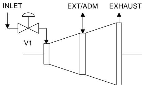
Steam can be extracted from or admitted to an extraction/admission turbine.
