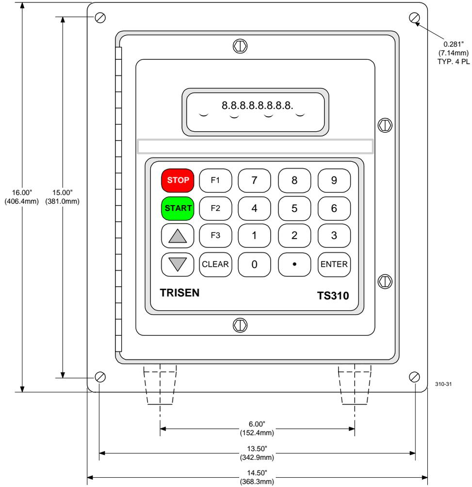
Figure 12. Flush Mounting Dimensions, Front View
