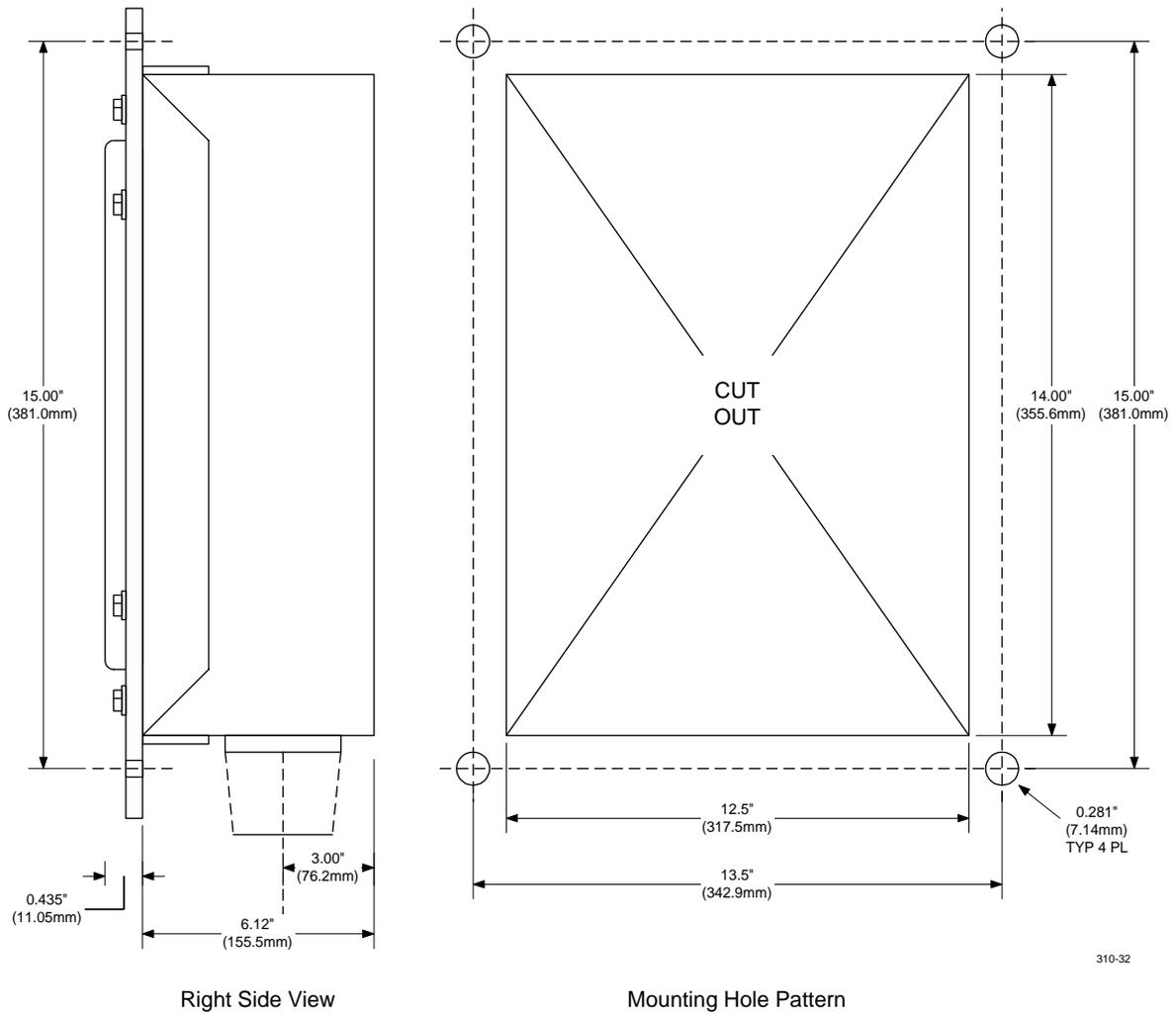
Figure 13. Flush Mounting Dimensions, Side View and Mounting Holes
