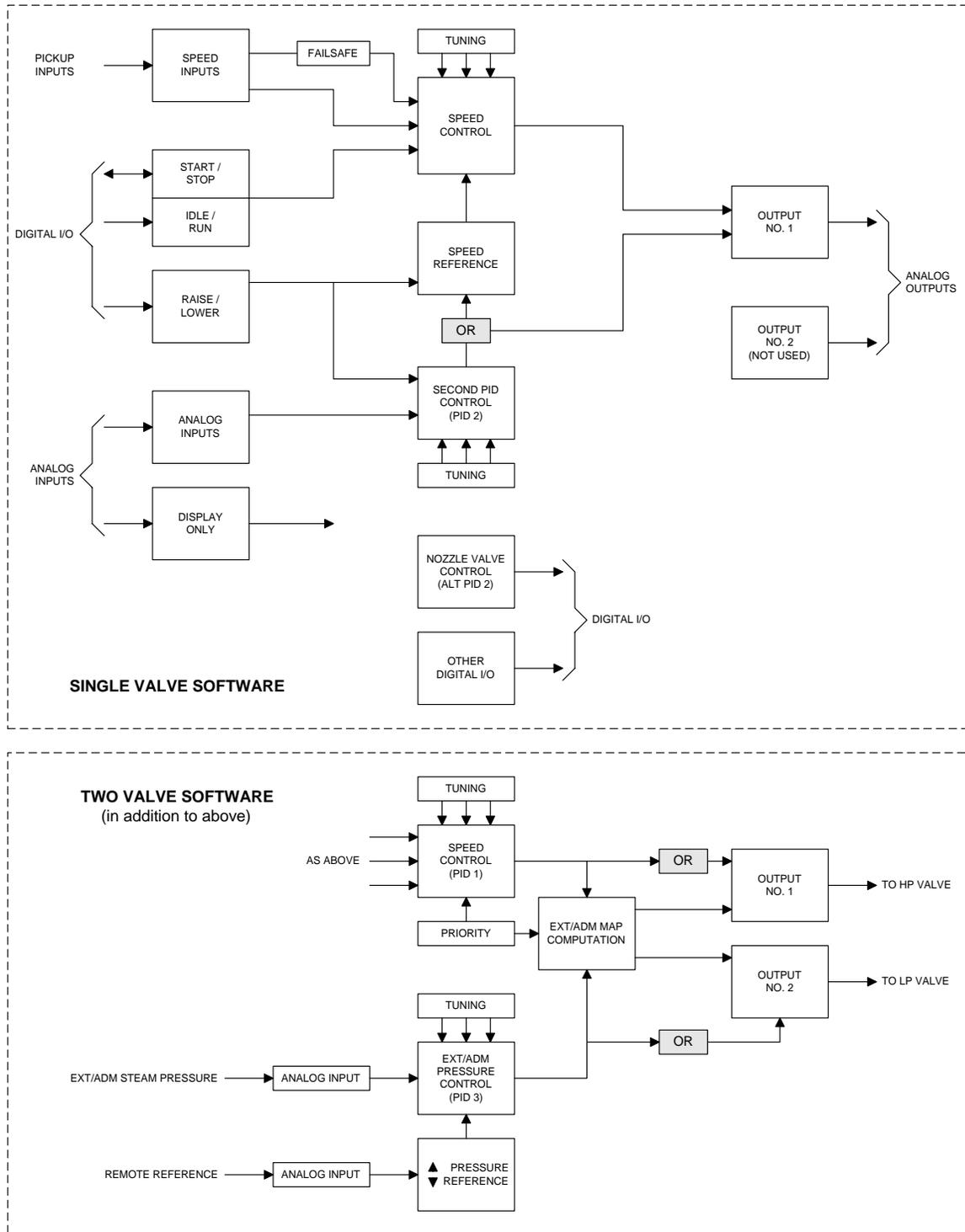
**Figure 2. TS310-02 Software Block Diagram**
