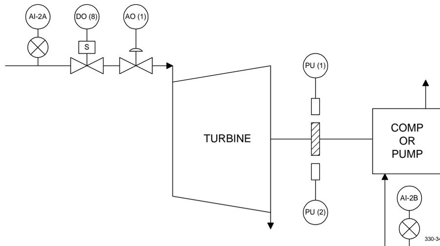
Figure 4. ACON.020 Inlet/Suction Pressure Control Typical Application
