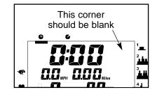
manual mode by pressing the Program button repeatedly until the upper right corner of the display is blank.
