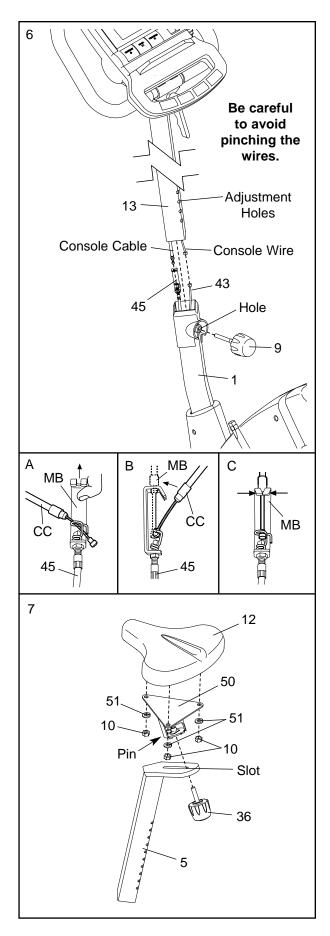
8. Turn the indicated Adjustment Knob (9) counterclockwise and remove it. Insert the Seat Post (5) into the Frame (1). Align one of the adjustment holes in the Seat Post with the indicated hole in the Frame. Insert the Adjustment Knob into the Frame and the Seat Post, and turn the Knob clockwise until it is tight. Make sure that the Knob is inserted through one of the adjustment holes in the Seat Post.
