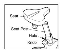
seat, first turn the indicated knob counterclockwise and remove it. Next, slide the seat post up or down and align one of the adjustment holes in the seat post with the indicated hole in the Frame. Insert the knob into the frame and the seat post, and turn the knob clockwise until it is tight. Make sure that the knob is inserted through one of the adjustment holes in the seat post.
