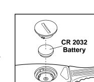
Remove the old battery and insert a new CR 2032 battery. Make sure that the battery is turned so the writing is on top. Replace the battery cover and turn it clockwise to close it.
