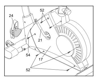
Turn the Crank (21) to the position shown. Using an adjustable spanner, turn the Left Pedal (24) clockwise and remove it. Next, remove the five M4 x 25mm Screws (52) and the M4 x 19mm Screw (54) from the Left Side Shield (17). Carefully remove the Left Side Shield.
