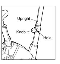
frame and the upright, and turn the knob clockwise until it is tight. Make sure that the knob is inserted through one of the adjustment holes in the upright.
