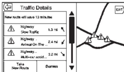
The detail view of the incident shows any data about the incident as well as how much time could be saved by avoiding it. The map view shows the incident, the original route, and the suggested route. If voice prompts are enabled, the incident information is spoken. Press the Take New Route screen button to change to the new route.
