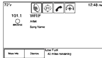
If the vehicle reaches a low fuel level, the system displays an alert about the low fuel condition. Press the More Info screen button to view nearby gas stations and start guidance, if desired.
