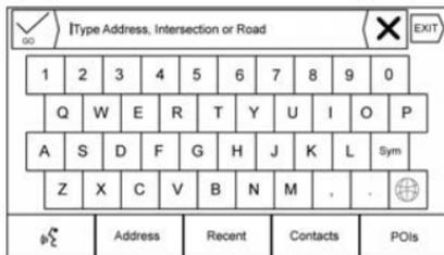
The keyboard is used in multiple locations throughout the system and can be used with many features. The navigation system uses the alpha-numeric system keyboard which includes 1 through 0, A through Z in QWERTY layout, hyphen, comma, period, Space, and Sym which would show additional characters needed.
