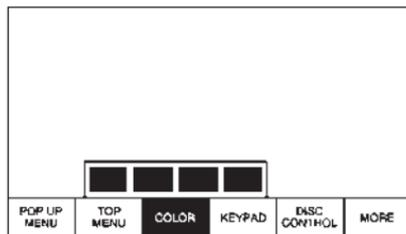
Select COLOR to display the four color button options: blue, yellow, red, and green. Highlight a color option and press ENTER and the appropriate action will be carried out. Press the Back button or MENU button, or wait for the 15-second time out to close the menu. Press the down arrow on the yellow color to keep the overlay menu up, but close the color menu. The color menu is disc dependent; selecting colors for discs that do not support this feature will have no function.
