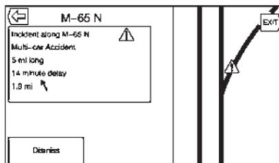
While driving and not under guidance, the system can receive data indicating an accident or slow traffic flow. The information about the incident or slow traffic is displayed as an alert when the incident is 5 km (3 mi) ahead. The incident can be viewed on the map. Press the Dismiss screen button to return to the previous map.
