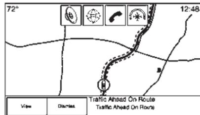
If data is received about a traffic development on the route ahead, a search for a better route is performed. If a better route is found, information may be displayed in an alert. This alert displays the route information and how much time may be saved. If the alternative route is accepted, the current route will be altered.
