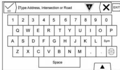
The keyboard may be able to perform an autocomplete function. Depending on the application, autocomplete matches entries that have been previously typed or are stored in a Recent Destinations list.
