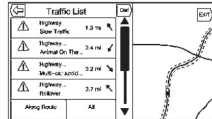
1. Press Show Nearby Traffic Incidents to access the Traffic List menu. This menu displays the incident symbol and highway name, along with the distance and heading to the incident.
