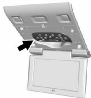
2. Move the screen to the viewing position. The remote must be removed from the storage location to be used.
