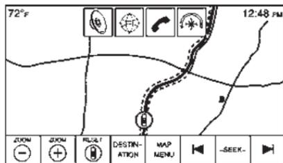
While at the Home Page, press the Nav screen button to display a view of the map. Press the Destination screen button to go to the destination entry views.
