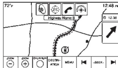
When driving in an area with no road showing on the map, the system transitions to off-road mode. The map displays a destination pointer in the Turn List area. The system will attempt to guide by showing a highlighted route starting at the nearest road. This road name is shown in the next maneuver name field at the top of the screen.
