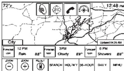
The weather application uses the navigation system to provide the appropriate information for the guidance route. When not under guidance, it defaults to the current location.
