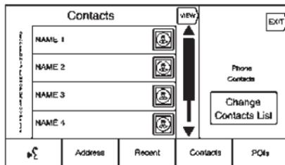
Select the Contacts button to view the vehicle's contact list or a connected Bluetooth device. Press the Change Contacts List screen button to switch between the vehicle's contact list and the Bluetooth device's contact list. If a particular contact has a single address associated with it, that contact has a Quick Route list item function button next to it. Contacts without this Quick Route button either have multiple addresses or no
