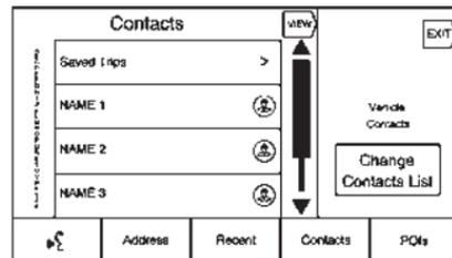
Trips from Contacts can be saved and recalled. The order is based on when the trip was last used. When the trips are saved, they are given a default title of the final destination name. If there are no saved trips, this list item is hidden.
