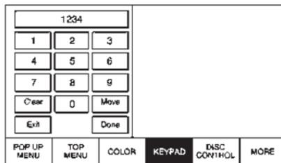
Press KEYPAD to display the single digit entry keypad. To close the keypad, press the Back button or MENU button, wait for the menu to time out, or press the down arrow to keep the menu up but close the keypad. The keypad is disc dependent; selecting numbers for discs that do not support this feature will have no function.
