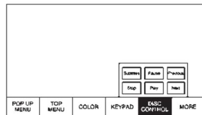
Press DISC CONTROL to display options for subtitles, play, pause, track forward, track previous, and stop the disc. Press the Back button or MENU button, or wait for the time out to close the menu. Press the down arrow from Stop, Play, or Next to keep the overlay menu up, but close the disc control menu. The disc control menu is disc
