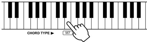
Pressing this key selects the major seventh chord type (M7). The display shows the name of the chord, and the individual notes — both in notation and on the keyboard diagram.
