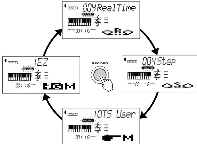
Each press of the RECORD button cycles through the four Record modes — Realtime, Step, OTS, and EZ Chord — before exiting back to normal operation. (The OTS and EZ Chord modes are unrelated to Song recording; they are described on pages 72 and 68, respectively.)
