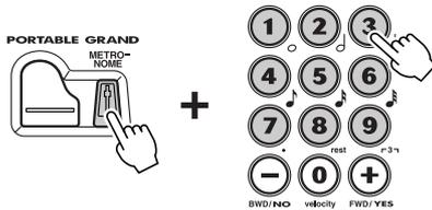
Normally, the Metronome is set to play in 4/4 time. To change this to 2/4, press number button "2." To change it to 3/4 time, press number button "3."
