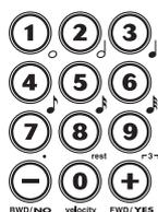
Style numbers can be selected in the same way as with the voices (see page 28). You can use the numeric keypad to directly enter the style number, use the +/- keys to step up and down through the styles, or press the STYLE button to advance through the style numbers.
