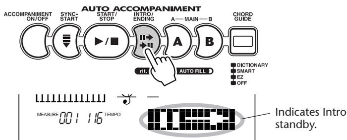
3) Press the SYNC-START button to enable Sync-Start, and start the Intro section and accompaniment by playing any key on the keyboard. (When auto accompaniment is on, play a key or chord in the auto accompaniment section of the keyboard.)
