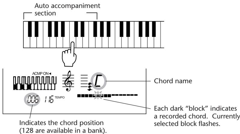
Each time you press a single key in the accompaniment section of the keyboard, EZ Chord plays the recorded chord and automatically advances to the next one. (Unrecorded "empty" blocks are skipped.) In this way, you can control the timing of chords with just a single finger of your left hand, and still use the powerful auto accompaniment features to create full backing — while you play melodies or solo with your right hand.
