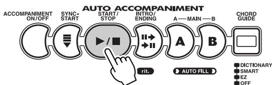
You can select the Main A or B section by pressing the appropriate button — MAIN A or MAIN B — before pressing the START/STOP button. (The icon section of the display briefly shows the letter of the selected section: “A” or “B.”)
