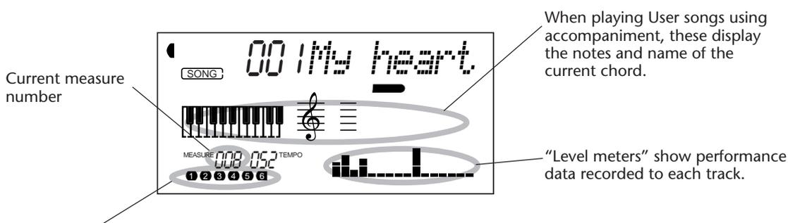
Indicates the tracks currently playing back. (These can be alternately muted and sounded during playback by pressing the corresponding SONG MEMORY buttons.)
