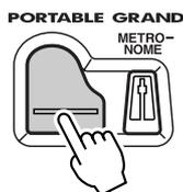
Doing this automatically cancels any other mode or function, and resets the entire instrument for playing the special “Stereo Sampled Piano” Grand Piano voice (voice 001). It automatically selects the Voice mode (with the Style mode active), and calls up style #91 (Rock-A-Ballad). It also resets the footswitch to Sustain operation.
