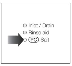
Fill the salt reservoir with dishwasher salt when the salt indicator light comes on. (If it comes on during a programme, wait until the end of the programme).
