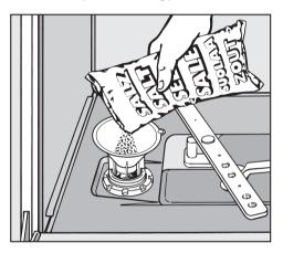
Place the funnel provided over the salt reservoir and carefully fill with salt until the reservoir is full. The salt reservoir holds approx. 2 kg of salt depending on the brand used.
