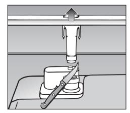
Cut off the top of the vent valve in the wash cabinet.
