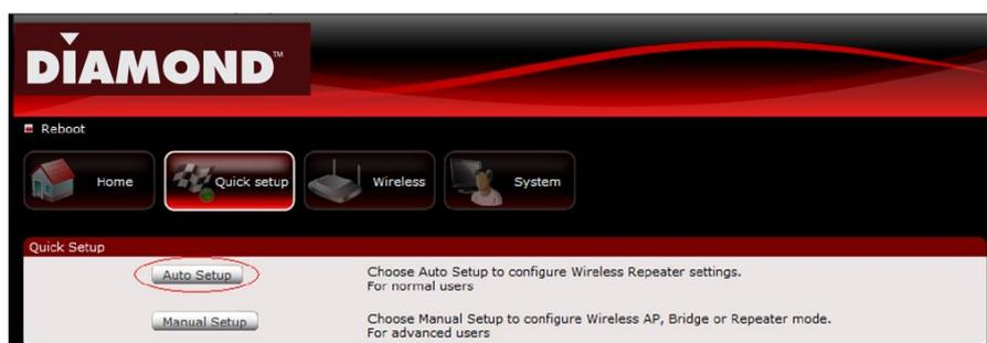
**NOTE:** If you are connecting to a hidden wireless network, you need to go through the Manual Setup and key-in the information from your existing wireless router/AP manually. Also un-tick the Broadcast SSID option so your wireless network can remain hidden.
