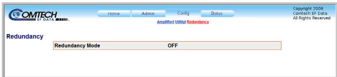
Redundancy page in Standalone Configuration (no redundant units recognized by system)
