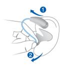
➤ For all other ear pieces: Grip the receiver in the ear canal with two fingers and pull it carefully out ②.
