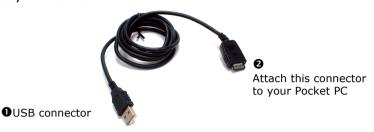
Attach the USB connector (①) to an available USB port of your PC and the ActiveSync® connector (②) to the ActiveSync® port of your Pocket PC. The PC must be switched on for charging through the ActiveSync® cable. Installing the included active-sync Software first before connecting the ActiveSync® cable!
