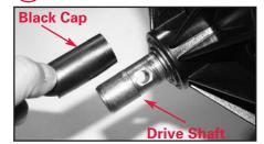
Collar bolt inserts into the large hole, passes through the drive shaft and threads into the small hole of the metal collar. Make sure bolt is tight. Some wiggle is normal between the power head and auger. Check and tighten often.
