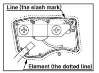
After cleaning, reassemble the air cleaner cover insert the tab at left, then insert the right tab and tighten fixing bolt
