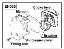
Dirty air cleaner element will cause starting difficulty, power loss, engine malfunctions, and shorten engine life. Keep the air cleaner element clean.
