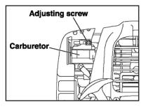
When the adjusting screw is turned right, engine rpm increases, and when it is turned left, rpm decreases. Never have auger rotation at idle.
