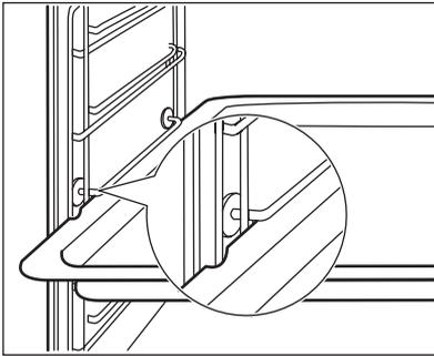
The deep pan and the wire shelf have side edges. These edges and the shape of the guide-bars are a special device to prevent the cookware from slipping.
