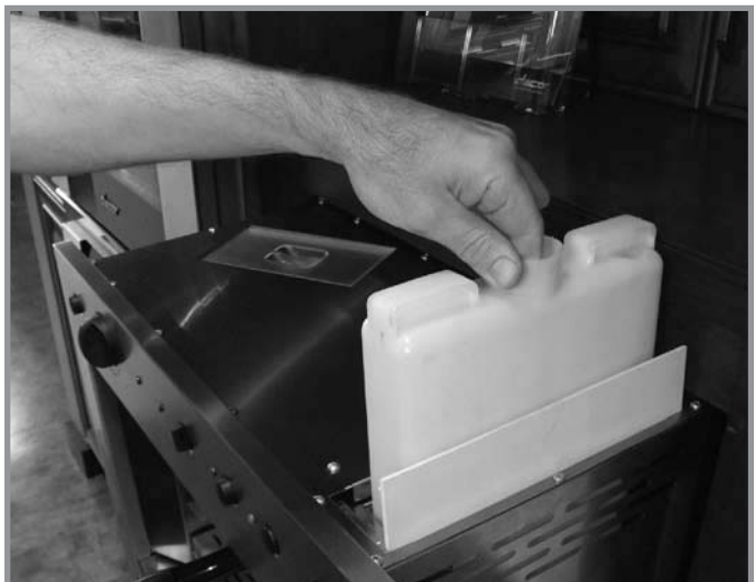
Water Tank Removal
