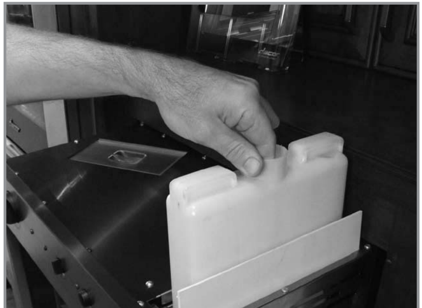
Removing the Water Tank
