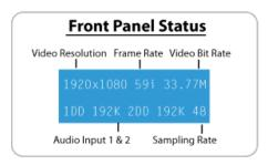
There are 9 menu trees accessible from the front panel. Using the **MODE** button, you can scan through the System, Decoder, Encoder, Transport, PID, Table, Profile, and Encryption menus. By pressing the **SELECT** button you can enter one of these sub menus.
