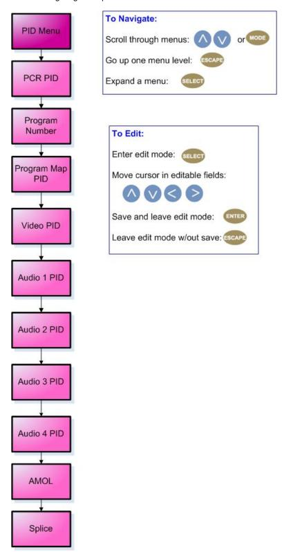
PCR PID Examples: PRP 1E1 (set the PID to 0x1e1 (481 decimal) PRP , 481 (set the PID to 481 (the comma is an empty placeholder) PRP 1E1 500 (set the PID to 500 (assumes 500 is different from the currently configured PID).
