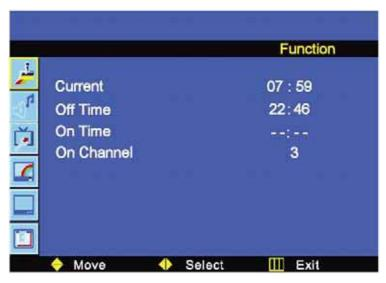
Press [▲] / [▼] to select different items, and press [▶] / [◀] to adjust Current, Off Time, On Time, and On Channel
