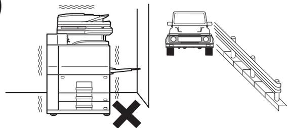
Vibration may cause failure.
