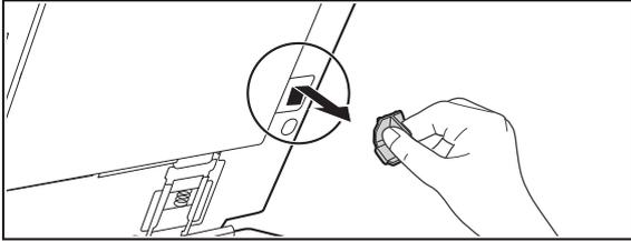
Open the automatic document feeder and remove the glass cleaner.
