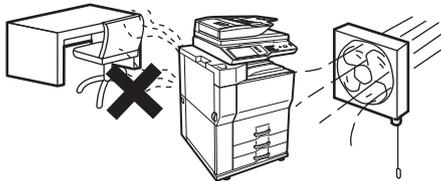
A small amount of ozone is created inside the machine during printing. The amount of ozone created is not sufficient to be harmful; however, an unpleasant odor may be noticed during large copy runs, and thus the machine should be installed in a room with a ventilation fan or windows that provide sufficient air circulation. (The odor may occasionally cause headaches.)
