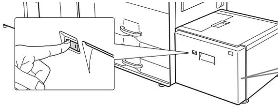
Press the operation button and wait until the operation button indicator turns off.
