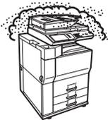
Risk of fire and electrical shock. If dust enters the machine, dirty output and machine failure may result.
