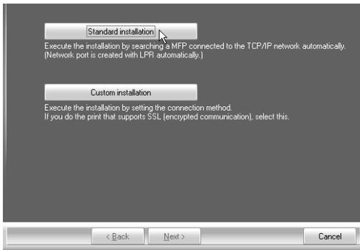
When [Custom installation] is selected, you can change any of the items below. When [Standard installation] is selected, the installation will take place as indicated below.
