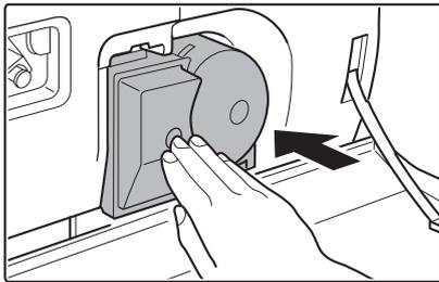
**Push the cartridge in until it locks securely in place.**
