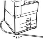
Placing heavy objects on the power cord, pulling it, or forcibly bending it will damage the cord, resulting in fire or electrical shock.
