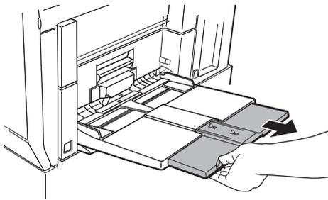
When loading 11" x 17", 8-1/2" x 14", 8-1/2" x 13", 8-1/2" x 11"R, A3, B4, or A4R size paper, pull out the tray extension.
