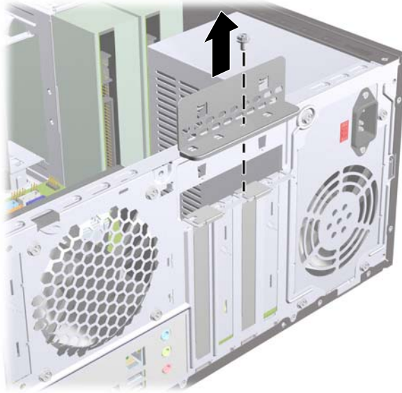
Figure 6-9 Opening the Slot Cover Lock
