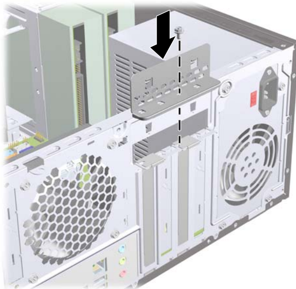
Figure 6-14 Securing the Expansion Cards and Slot Covers
