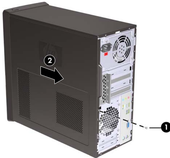
Figure 6-1 Removing the Computer Access Panel
