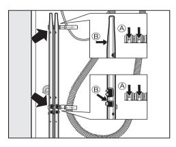
■ Secure the transit bars to the back of the machine. Make sure that holes <sup>®</sup> are fitted over retainers <sup>A</sup>.
