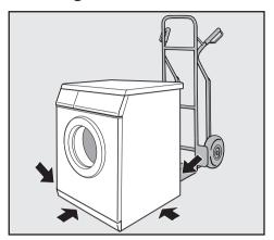
■ Remove the packaging and position the machine where you want to use it.
