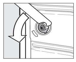
■ Using the notched end of the spanner supplied, turn the left-hand transit bar 90°. then
