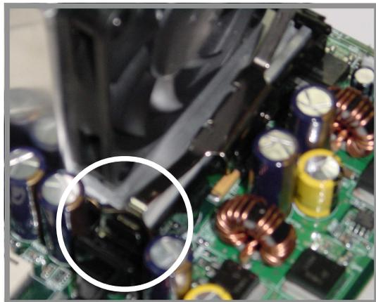
3. Use a small flat screw driver to attach the other end of the bracket, while firmly holding down the heatsink and fan assembly. The middle hook of the bracket snaps in place if you properly attached the two ends.
