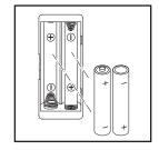
In case of a power failure, the appliance relies on battery backup. For this purpose, the appliance uses two batteries (AAA). The appliance remembers the time, but does not display it.
