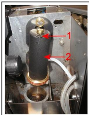
Carefully press the lubricant into the 2 points shown where the square block goes into the machine. Jiggle the block with your hand while working the lubricant in for better coverage and then re-assemble.
