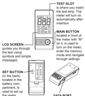
**DATA PORT** located at the side, is for cable connection.
