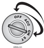
Turn ignition to the “on” position and then to the “off” position. Press and release the Valet® switch within 10 seconds. The status LED will light solid if you have entered Valet® Mode. The LED will turn off when exiting Valet® Mode.
