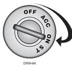
Turn the ignition on. Press and release the Valet® switch within 10 seconds. The LED will stop flashing and the vehicle should start. If it does not start, you may have waited too long. Turn the ignition off and try again.
