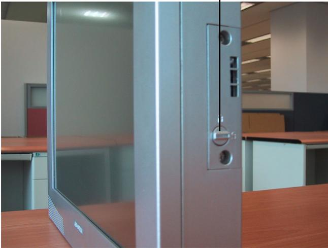
**Figure 2.6: Power switch in lock status**
