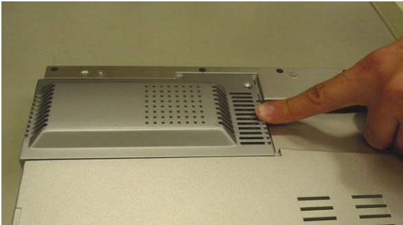
**Figure 3.3: Detaching the CPU plastic cover and heat sink**
