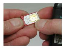
The cell phone has a SIM Card holder with two wedges; place the SIM Card in between the two wedges and the holder.
