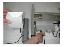
Plug the cable of the rain collector into the female plug called "**Regen**". By easily turning the audio connector, the plug snaps into place.
