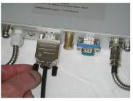
The black cell phone cable with the 9 pole plug should be plugged into the case where it is labeled "Handy" CAUTION:
