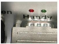
The LED blinks green during the Test SMS, and blinks red if there is an error. See the error code in the label..
