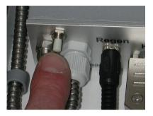
A Test-SMS is started when the pushbutton is pushed and held down for 3 seconds.
