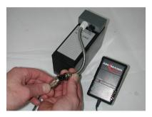
And when the red LED on the battery charger lights up, the accumulator cable fits correctly. The head of the plug must fit the counterpart.
