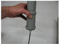
The plastic tube with the cell phone in place should hang so that the cable and the cable screw always face down.
