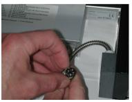
Connect the cable of the accumulator to the scale. Make sure that the head of the plug faces down, only then does it correctly make contact.
