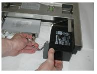
Lay the accumulator in the provided compartment.
