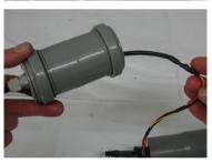
The cable is provided with a cable header so that the cable screw correctly prevents moisture.
