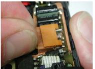
Make sure that the brown plug in on the board is fully clicked into place.
