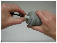
First, unscrew the cable screw so that air can enter.
