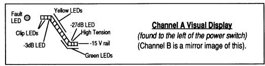
A simple, yet thorough, Visual display section is found on the Front Panel of the amplifier. This section provides the user with the necessary day-to-day function of an Output Level LED Ramp, as well as including various circuitry status indicators.
