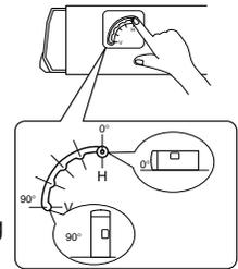
Be sure to apply the cover labels after setting the position of the springs so as to protect the interior of the product from dust or dirt which may cause malfunction.
