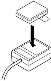
**2** Before completing the sensor mounting, make sure the location selected is within the operating range of the remote control. Peel off the backing of the adhesive tape and press the sensor onto the selected mounting location, or inside of the remote control holder.
