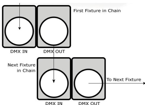
**A quick note:** Often, the setup for Master-Slave and Standalone operation requires that the first fixture in the chain be initialized for this purpose via either settings in the control panel or DIP-switches. Secondly, the fixtures that follow may also require a slave setting.
