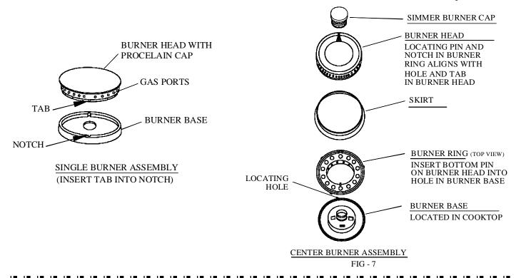
CAUTION: IMPROPER POSITIONING OF BURNER CAN DAMAGE COOKTOP AND CAUSE INJURY TO PERSONS.
