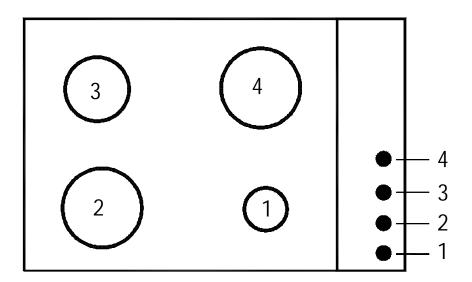
1 – Right Front Burner Control 9,000 BTU/HR 2 – Left Front Burner Control 15,000 BTU/HR 3 – Left Rear Burner Control 12,000 BTU/HR 4 – Right Rear Burner Control 15,000 BTU/HR
