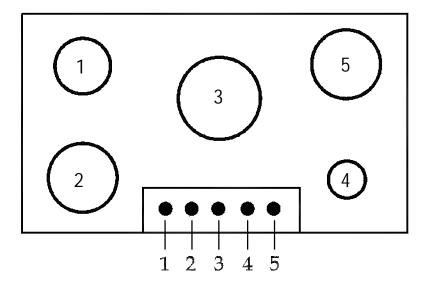
1 – Left Rear Burner Control 12,000 BTU/HR 2 – Left Front Burner Control 15,000 BTU/HR
