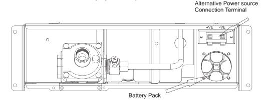
If you wish to connect your outdoor fire to mains electricity instead of using 3x D sized batteries, you may do so using the Alternative Power Source Connection Terminal, located on the control tray above the battery pack, as shown above.
