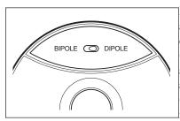
In Dipole mode the 8200 SR and 6200 SR produce ambience with minimal localization (best for most movies and video soundtracks) and more localizable sound in the Bipole mode (preferred for some music recordings). Switching between Dipole
