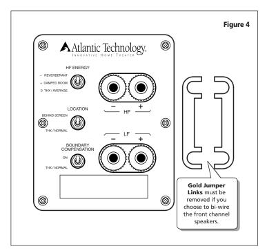
You can Bi-Wire by connecting two sets of speaker wires from the amplifier terminals to the input terminals on the back of the speaker enclosure. The wires should be attached to a single output terminal set on the amplifier. The other end is attached to the two sets of input terminals on the rear panel of the loudspeaker. Some manufactured Bi-Wire cables have only a single set of connectors at the amplifier end and two sets of connectors at the speaker end.
