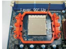
STEP 1: Lift Up The Socket Lever
