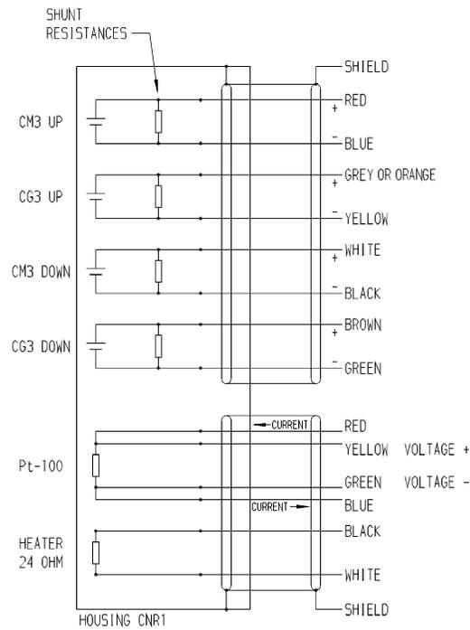
FIGURE 5-1. CNR1 Schematic
