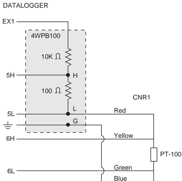
FIGURE 5-2. Interfacing the Pt-100 Using the 4WPB100 Module
