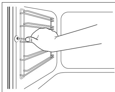
2. Pull the shelf support from the back of the side wall to remove it.
