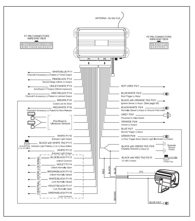
**NOTE:** The current draw for the entire security system when in the armed state is 20mA. Power supply voltage range is 9 volts to 15 volts.
