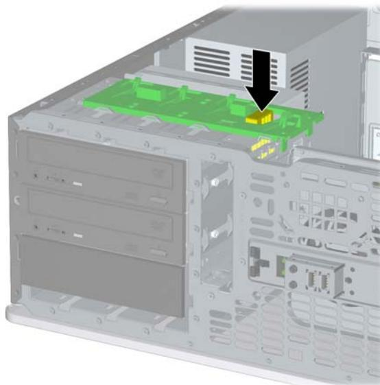
6. Before you reinstall each drive into the chassis, turn it so that it is in the same orientation as the internal 3.5-inch drive. The bottom of the drive should be parallel to the yellow drivelock.
