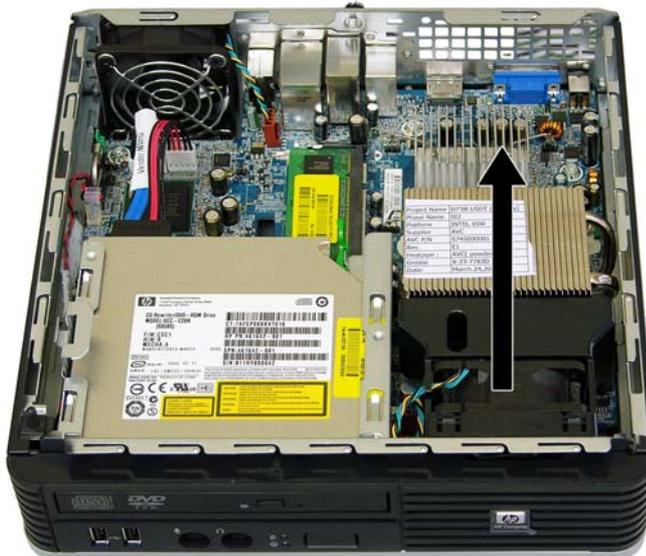
To install the front fan, reverse the removal procedure.
