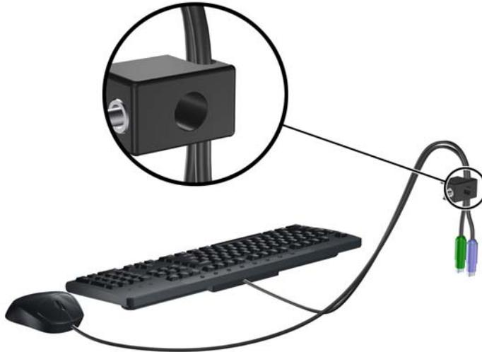
3. Screw the lock to the chassis using the screw provided.
