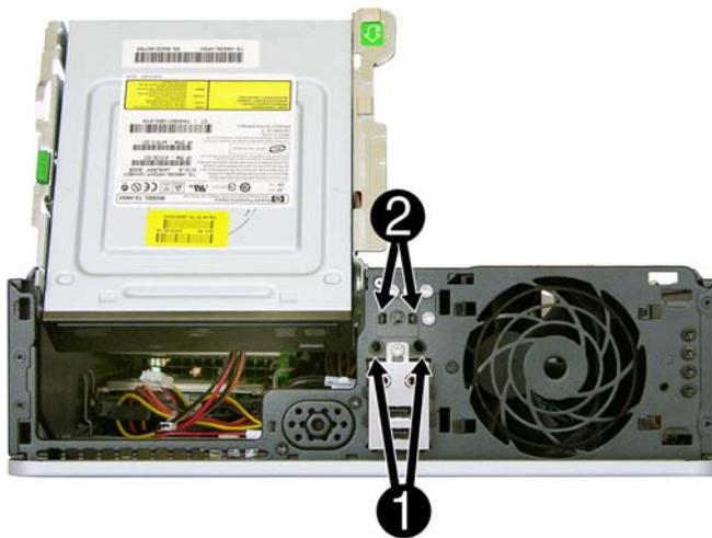
9. Lift the assembly up and out of the chassis, threading the wires through the hole in the drive cage bracket.
