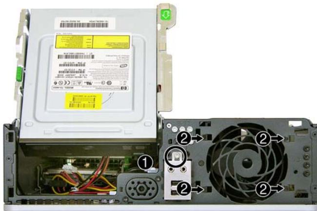
To install the chassis fan, reverse the removal procedure. Be sure to orient the air flow into the unit.
