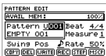
2. Use [CURSOR] to move the cursor to Pattern, then select "P001" – "P296" with the TIME/VALUE dial. You can press [PLAY] at this time to hear the selected preset rhythm pattern. Press [STOP] to stop the performance.
