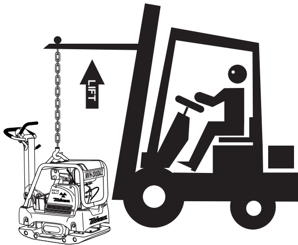
Figure 18. Lifting the Compactor
