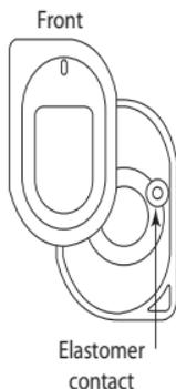
**Note:** Make sure that the small elastomer contact located inside the unit as shown does not fall out during the replacement process.
