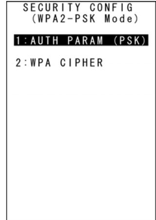
2. Use the cursor keys ([▲] [▼]) or numerical key ([1]) to highlight [1: AUTH PARAM (PSK)] and then press the **ENT** key.
