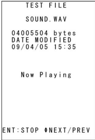
Use the cursor keys ([◀] [▶]) to adjust the volume. The volume can be adjusted in four levels from 0 (minimum) to 3 (maximum.)
