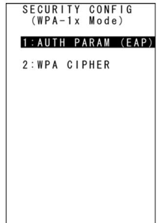
2. Use the cursor keys ([▲] [▼]) or numerical key ([1]) to highlight [1: AUTH PARAM (EAP)] and then press the **ENT** key.
