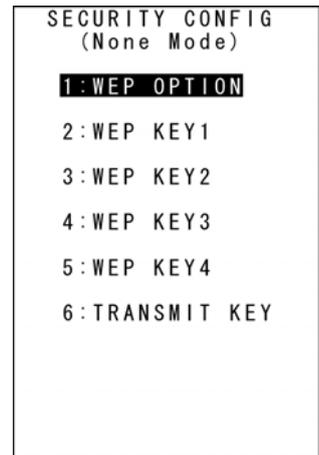
2. Use the cursor keys ([▲] [▼]) or numerical key ([1]) to highlight [1: WEP OPTION], and then press the **ENT** key.
