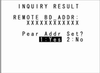
If the detected device does not exist, the screen on the right is displayed.
