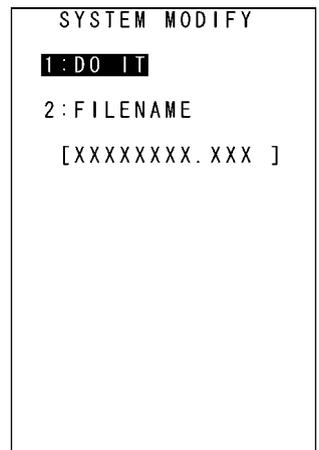
2. Use the cursor keys ([▲] [▼]) or numerical key ([1]) to highlight [1: DO IT] and then press the **ENT** key.
