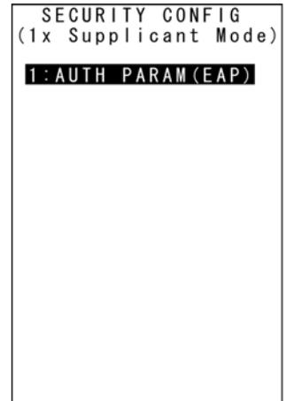
2. Ensure that [1: AUTH PARAM (EAP)] is highlighted and then press the **ENT** key.
