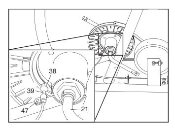
Next, turn the resistance knob to the lowest setting. With the left shield removed, locate the Reed Switch (39). Turn the Crank (21) until the Magnet (38) is
