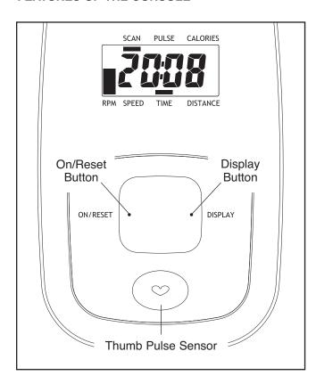
The console offers a selection of features designed to make your workouts more effective. As you pedal, the console will provide continuous exercise feedback. You can even measure your heart rate using the built-in thumb pulse sensor.
