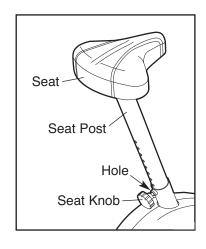
or downward and align one of the adjustment holes in the seat post with the indicated hole in the frame. Then, insert the seat knob into the frame and the seat post, and turn the seat knob clockwise until it is tight. Make sure that the seat knob is inserted through one of the adjustment holes in the seat post.
