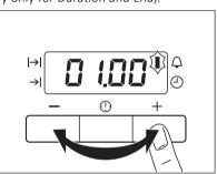
With the functions Duration  $\rightarrow$  and End  $\rightarrow$  the oven stops automatically.
