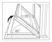
The oven door has 2, 3 or 4 panels of glass (depends on the model)
