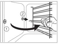
Installing the shelf support rails Install the shelf support rails in opposite sequence.
