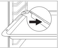
Inserting the oven shelf and deep roasting pan together
