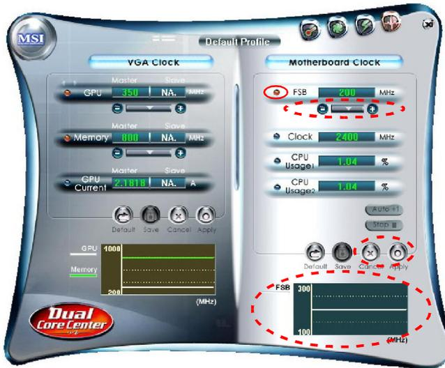
On the underside, it shows the graphs of the clocks. Only the curves of the item which the button is lit up with red color will be shown.
