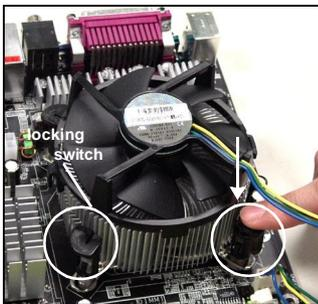
12. Turn over the mainboard to confirm that the clip-ends are correctly inserted.
