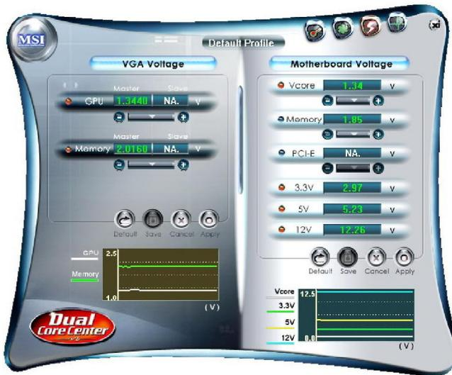
On the underside, it shows the graphs of the voltages. Only the curves of the item which the button is lit up with red color will be shown.
