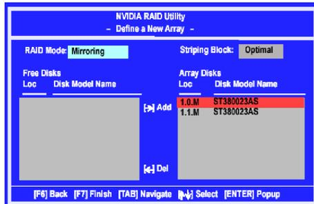
It shows that two disks have been assigned as RAID1 array disks in the figure above.
