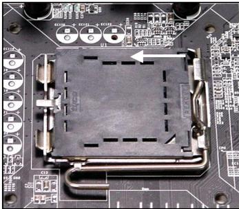
2. Remove the cap from lever hinge side (as the arrow shows).
