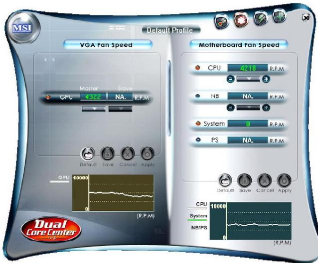
On the underside, it shows the graphs of the fan speed. Only the curves of the item which the button is lit up with red color will be shown.
