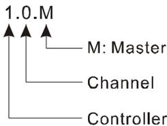
In the example above, 1.0.M means the hard drive is attached to Controller 1, Channel 0, and the drive is set to Master. The following is a list of all possible combinations:
