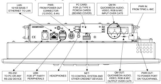
When connecting power, Crestron recommends using the included TPMC-L-IMC Interface Module to bring power from the included power supply to the touchpanel. The TPMC-L-IMC is connected between the power supply and touchpanel and allows power lines to be run from a remotely located power supply to the touchpanel using 14 gauge stranded speaker wire as shown in the following diagram.
