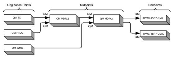
The TPMC-15/17-QM-L is not a switcher, but a transmitter/endpoint. Therefore, even when designated as the endpoint from two midpoint switchers, the QM output of the TPMC-15/17-QM-L can become another transmitter sending RGB video at the touchpanel's native resolution and aspect ratio. Refer to the following diagram.
