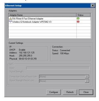
To configure the Ethernet adapter, click once on its name to select it in the *Adapter Name* list. Then, click **Configure** to open the "EthernetExternal Properties" window. This window displays the connection and related required items.
