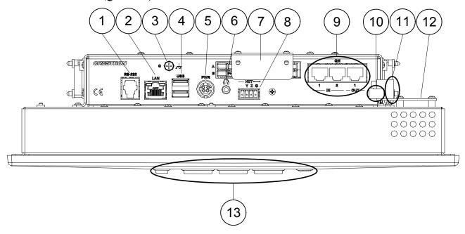
**NOTE:** Connectors on the TPMC-15/17-L CH version are identical to those on the QM version except for item number 9 above. The CH version, has **Video IN** and **Audio I/O** ports instead of the **QM IN** and **QM OUT** ports.
