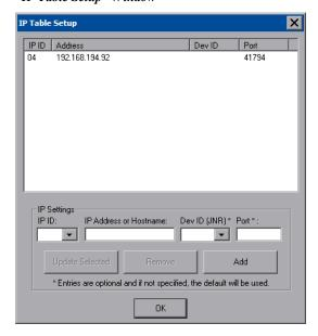
The IP ID is the ID number that is used to identify the touchpanel in the control system's IP table. The IP ID should match the IP ID set in the SIMPL Windows program.
