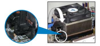
3. When the fan and heatsink assembly is in place, connect the CPU fan cable to the connector on the motherboard labeled CPU\_FAN.
