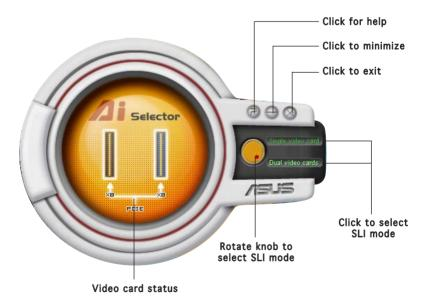
**Single Video Card mode** - the primary (blue) PCI Express x16 slot works at the bandwidth of PCI Express x16.
