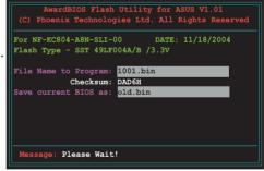
4. The utility saves the current BIOS file to the floppy disk, then returns to the BIOS flashing process.
