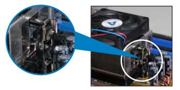
3. Align the other end of the retention bracket (near the retention bracket lock) to the retention module base. A clicking sound denotes that the retention bracket is in place.
