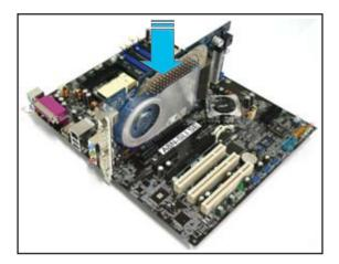
4. Insert the second graphics card into the black slot labeled PCIEX16\_2. Make sure that the card is properly seated on the slot.
