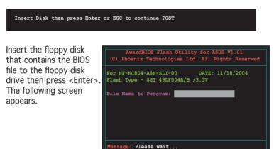
5. When the correct BIOS file is found, EZ Flash performs the BIOS update process and automatically reboots the system when done.
