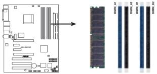
A8N-SLI SE 184-pin DDR DIMM Sockets
