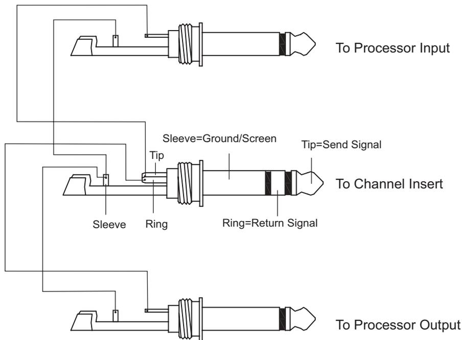
**Y -Stereo lead for insert Connection**
