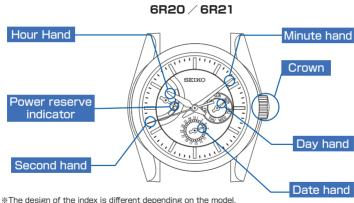
\* The design of the maex is different depending on the model
