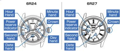
\* The design of the index is different depending on the model.
